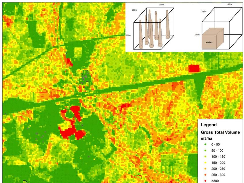
LiDAR's ability to detect three-dimensional objects helps planners accurately calculate timber volumes and areas of density. In the heat map above, orange and red areas indicate timber volumes greater than 200 cubic metres per hectare.
