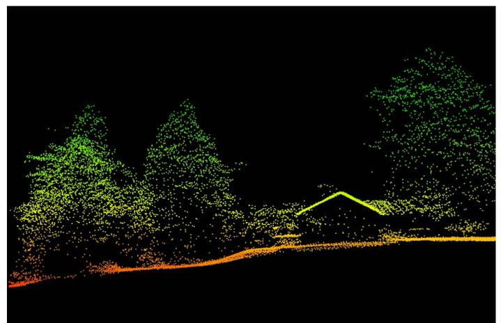
Cross-section view of LiDAR point cloud showing tree, topography and terrain details.
